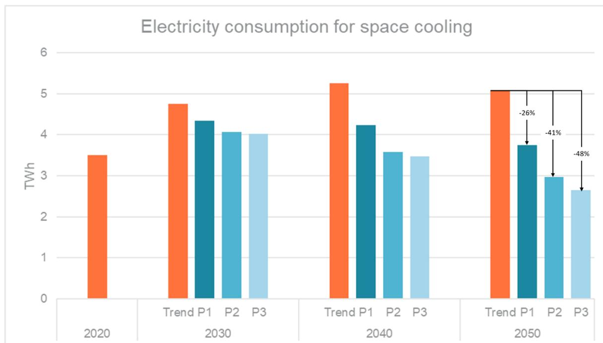
**Figure 5** Mitigation prospects - Electricity consumption for space cooling 2020 - 2050
