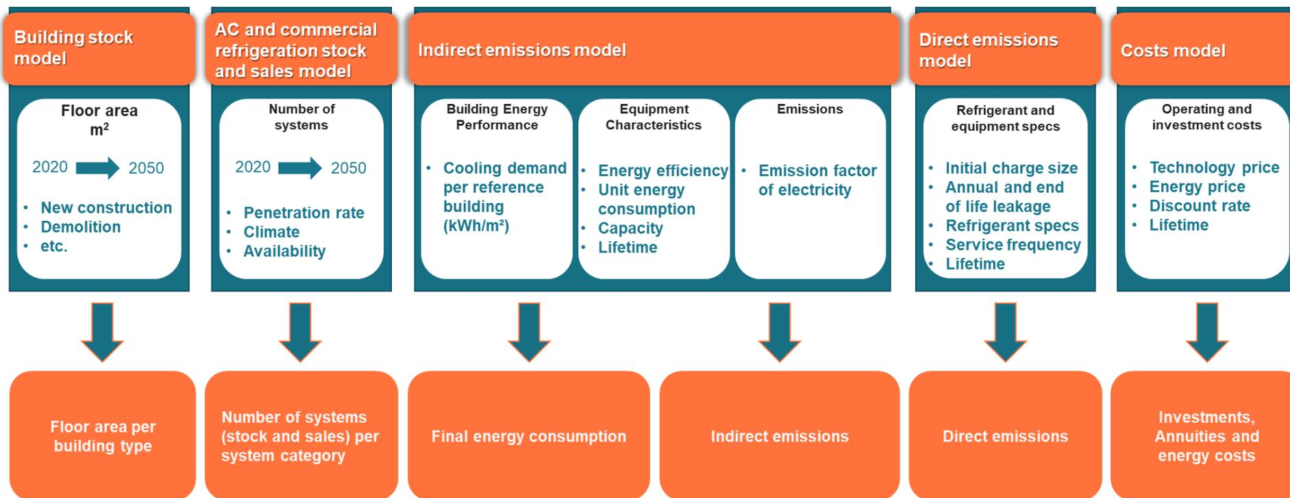
**Figure 1** Calculation methodology, models, and corresponding outputs
