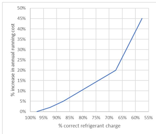
**Figure 3** Relationship between Annual running costs and refrigerant leakage for small air-conditioning and commercial systems.<sup>37</sup>
